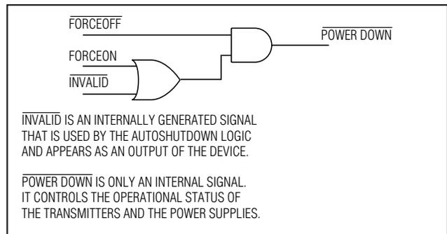
Figure 3c. AutoShutdown Logic
