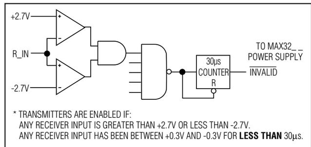
Figure 3b. MAX3221/MAX3223/MAX3243 with Transmitters Enabled Using AutoShutdown
