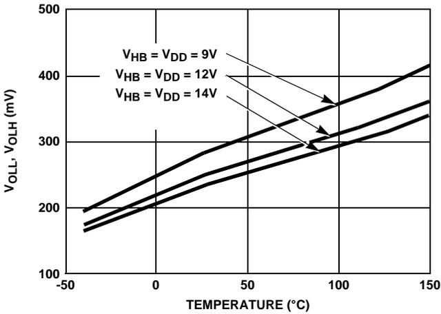
FIGURE 8. LOW LEVEL OUTPUT VOLTAGE vs TEMPERATURE
