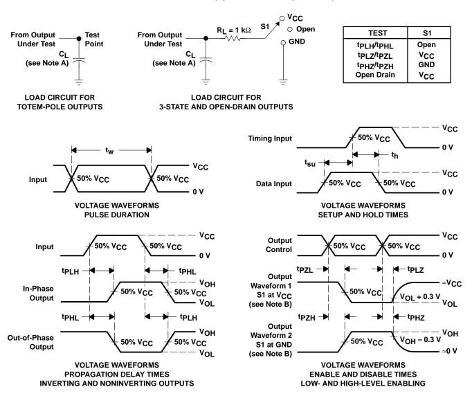
NOTES: A. C<sub>L</sub> includes probe and jig capacitance.
