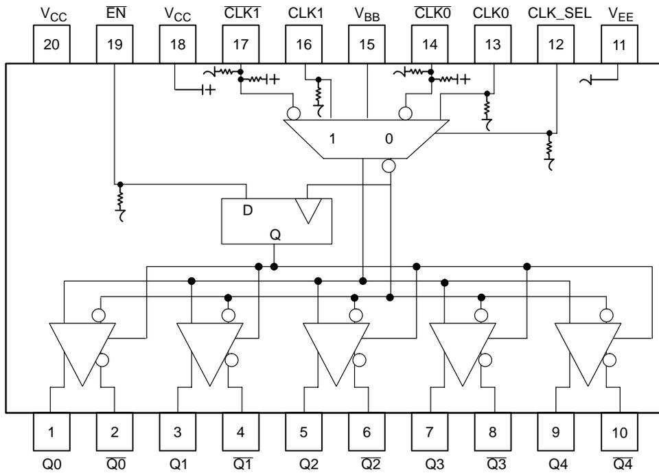
Warning: All  $V_{CC}$  and  $V_{EE}$  pins must be externally connected to Power Supply to guarantee proper operation.
