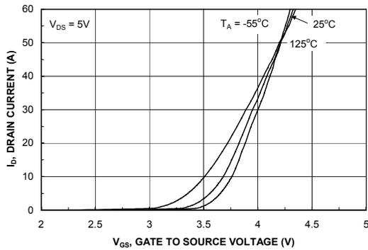
Figure 5. Transfer Characteristics.
