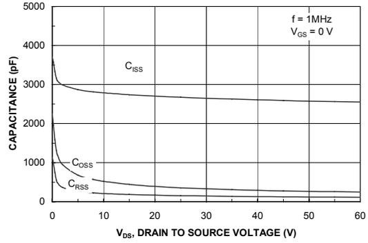
Figure 8. Capacitance Characteristics.
