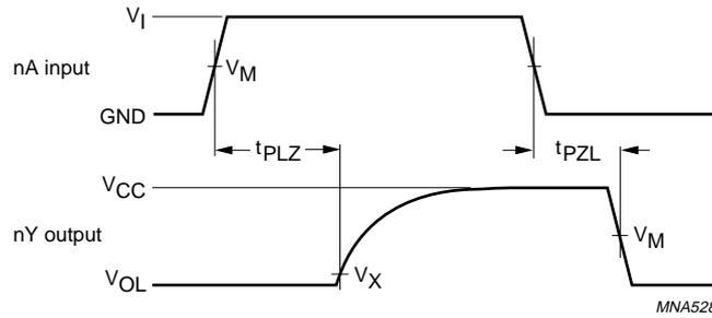
For 74HC3G07:  $V_M = 50\%$ ;  $V_I = \text{GND to } V_{CC}$ .
