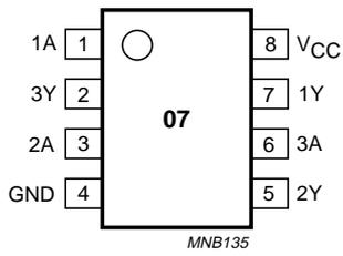
Fig.1 Pin configuration.
