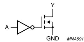
Fig.4 Logic diagram (one driver).
