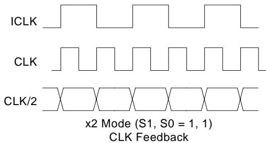
Using CLK as the feedback will always result in synchronized rising edges between ICLK and CLK. However, the CLK/2 could be a falling edge compared with ICLK. ICS recommends using CLK/2 feedback whenever possible. This will synchronize the rising edges of all three clocks.
