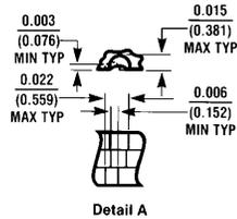
**20-Lead Ceramic Leadless Chip Carrier (L)**
