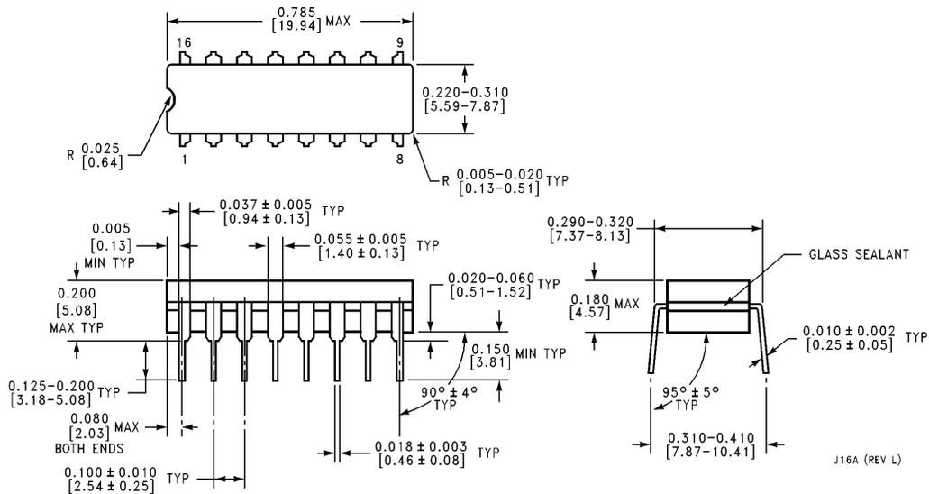
**16-Lead Ceramic Dual-In-Line Package (D)**
