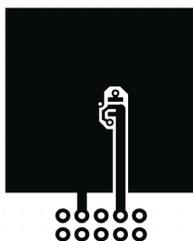
a)  $78^\circ\text{C}/\text{W}$  when mounted on a  $1\text{ in}^2$  pad of 2 oz copper
