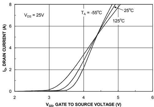
Figure 5. Transfer Characteristics.
