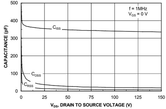
**Figure 8. Capacitance Characteristics.**
