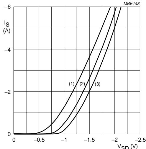
Fig.8 Source current as a function of source-drain diode forward voltage.
