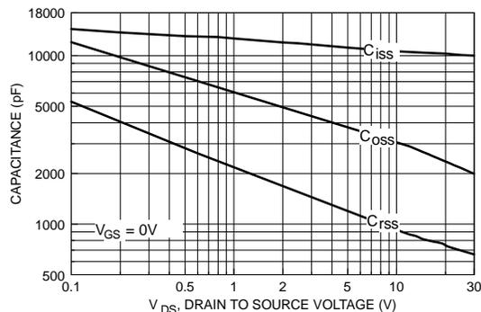
Figure 8. Capacitance Characteristics.
