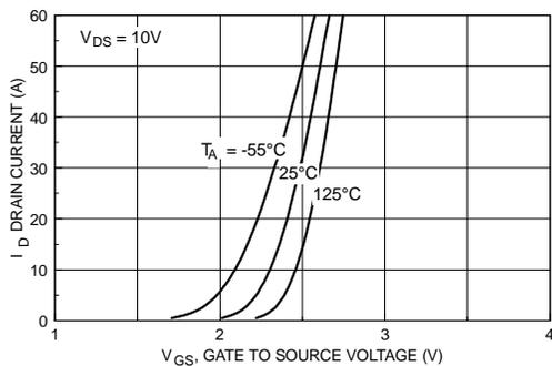
Figure 5. Transfer Characteristics.
