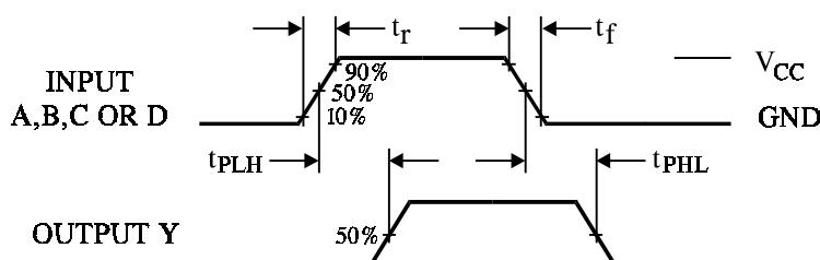
Figure 1. Switching Waveforms
