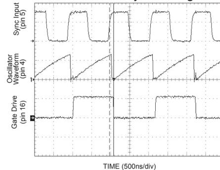
Figure 6. Sync Waveform
