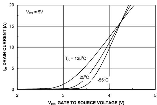
Figure 5. Transfer Characteristics.
