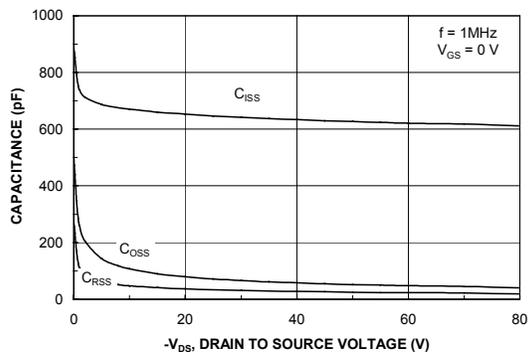
Figure 8. Capacitance Characteristics.
