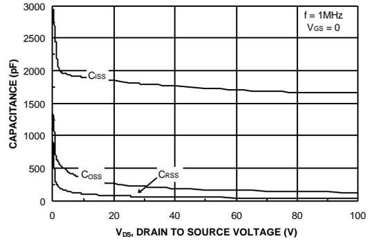
Figure 8. Capacitance Characteristics.
