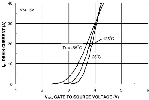
Figure 5. Transfer Characteristics.
