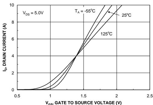
Figure 5. Transfer Characteristics.
