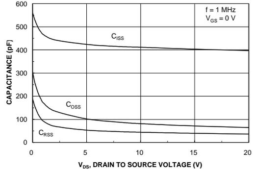
Figure 8. Capacitance Characteristics.
