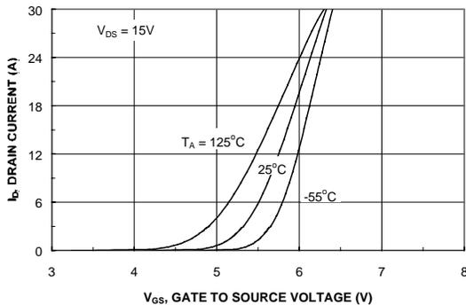
Figure 5. Transfer Characteristics.
