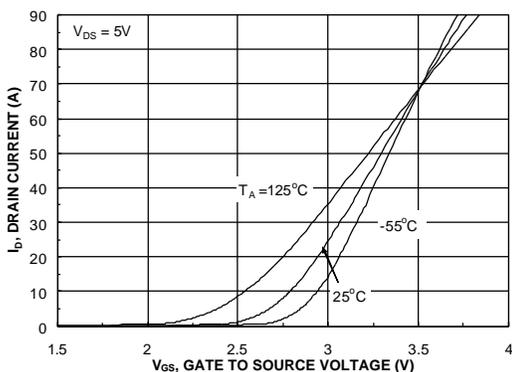
Figure 5. Transfer Characteristics
