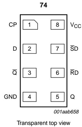
Fig.2 Pin configuration XSON8.
