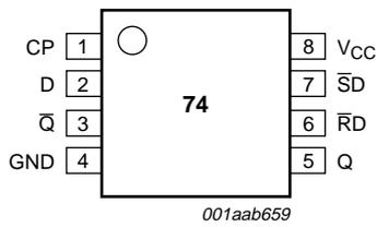
Fig.1 Pin configuration TSSOP8 and VSSOP8.
