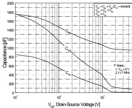
**Figure 5. Capacitance Characteristics**
