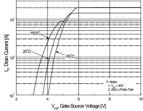
**Figure 2. Transfer Characteristics**
