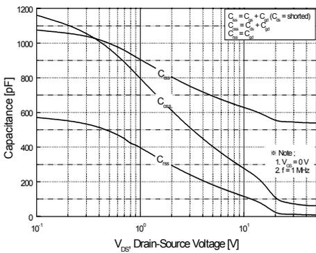
Figure 5. Capacitance Characteristics
