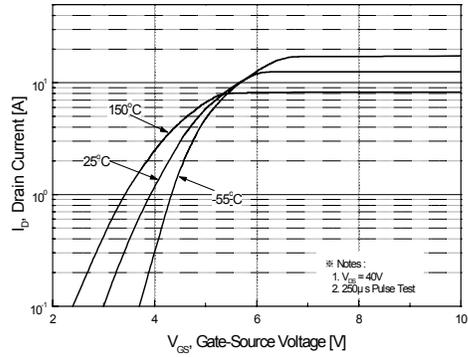
Figure 2. Transfer Characteristics
