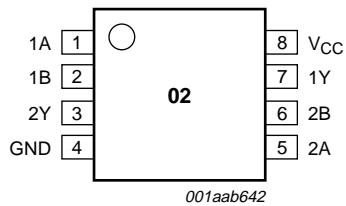
Fig.1 Pin configuration TSSOP8 and VSSOP8.
