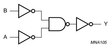
Fig.5 Logic diagram (one gate).
