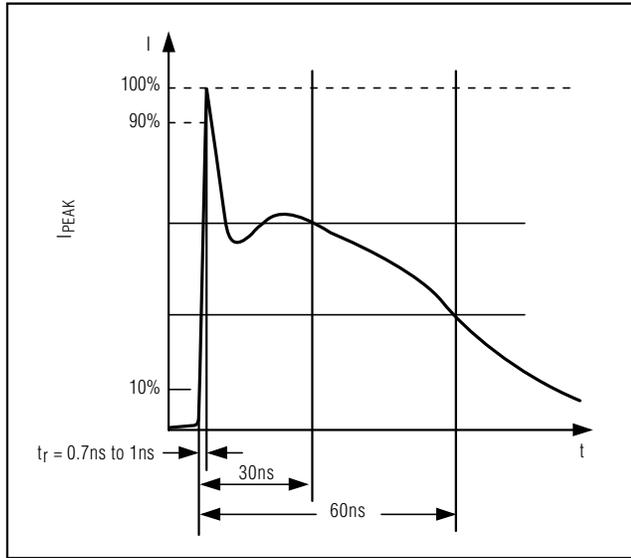
Figure 6b. IEC 1000-4-2 ESD Generator Current Waveform
