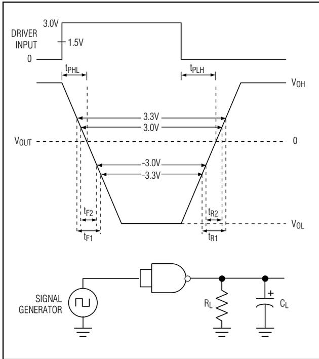
Figure 1. Slew-Rate Test Circuit and Timing Diagram
