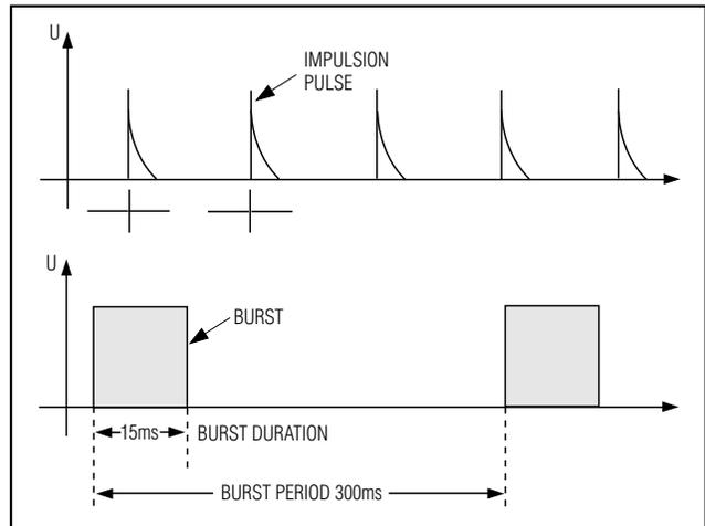
Figure 5. General Graph of a Fast Transient Burst
