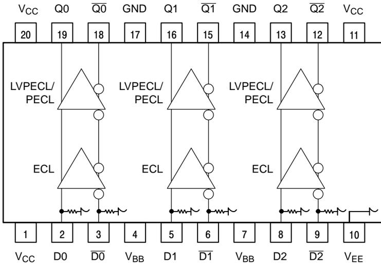
**Warning:** All  $V_{CC}$ ,  $V_{EE}$  and GND pins must be externally connected to Power Supply to guarantee proper operation.
