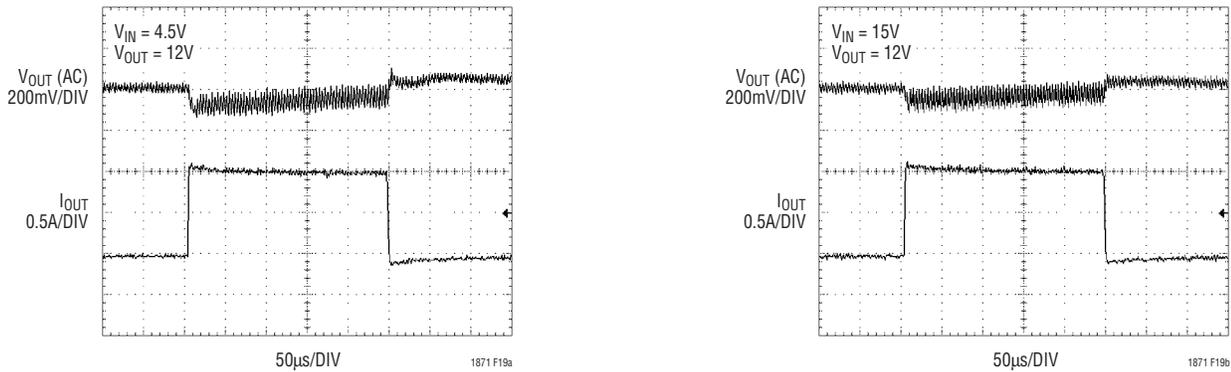
Figure 19. LTC1871 SEPIC Converter Load Step Response
