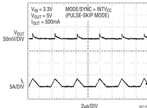
Figure 4. LTC1871 Low Output Current Operation with Burst Mode Operation Disabled (MODE/SYNC = INTV<sub>CC</sub>)
