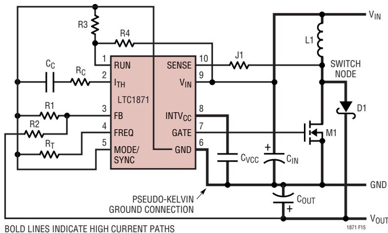
Figure 15. LTC1871 Boost Converter Layout Diagram
