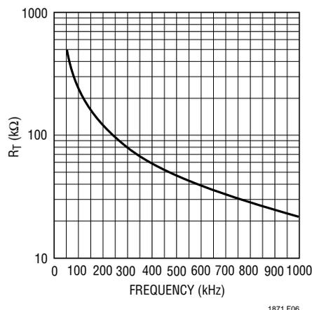
Figure 6. Timing Resistor ( $R_T$ ) Value
