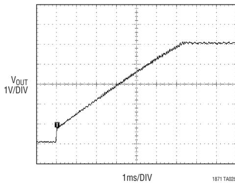
Load Step Response at  $V_{IN} = 4.5V$
