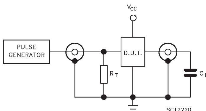
C<sub>L</sub> = 15/50 pF or equivalent (includes jig and probe capacitance)R<sub>T</sub> = Z<sub>out</sub> of pulse generator (typically 50Ω)
