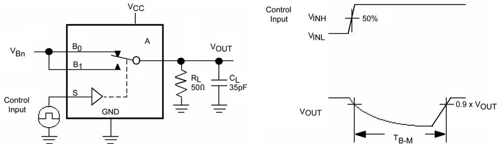
$C_L$  Includes Fixture and Stray Capacitance
