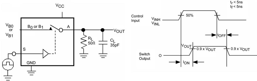
$C_L$  Includes Fixture and Stray Capacitance
