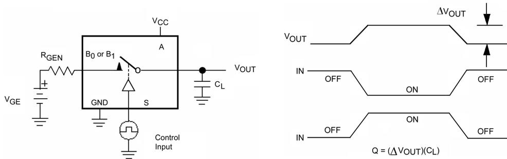
**FIGURE 4. Charge Injection**
