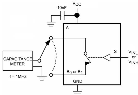
**FIGURE 5. ON/OFF Capacitance Measurement Setup**
