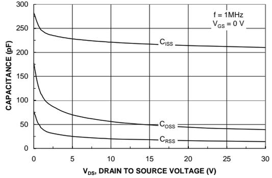
Figure 8. Capacitance Characteristics.
