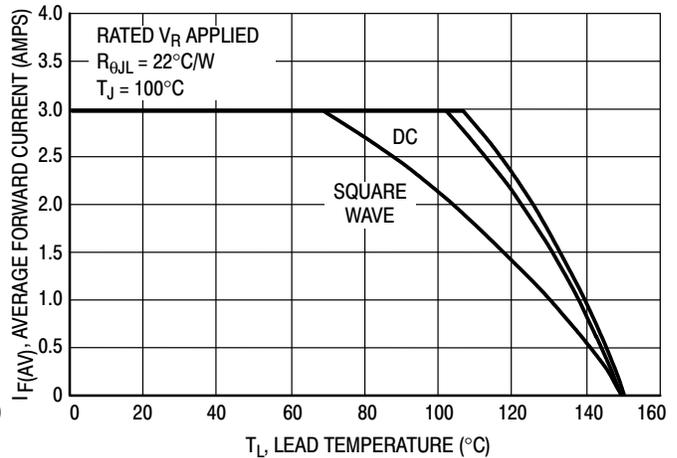
Figure 4. Current Derating, Lead
