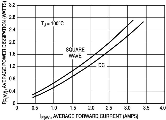
Figure 3. Power Dissipation
