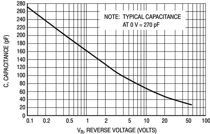
Figure 5. Typical Capacitance
