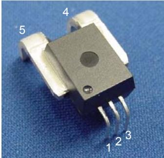
Pin 1:  $V_{CC}$       Terminal 4:  $I_{p+}$
