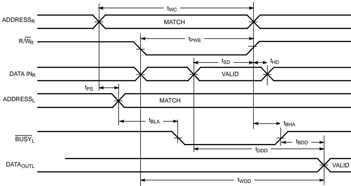
**Write Timing with Busy Input ( $\overline{\text{M/S}}=\text{LOW}$ )**
