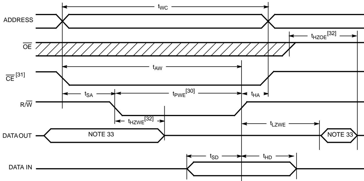
**Write Cycle No. 2: CE Controlled Timing<sup>[27, 28, 29, 34]</sup>**
