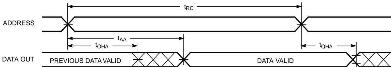
**Read Cycle No. 2 (Either Port  $\overline{CE}/\overline{OE}$  Access)**<sup>[22, 25, 26]</sup>
