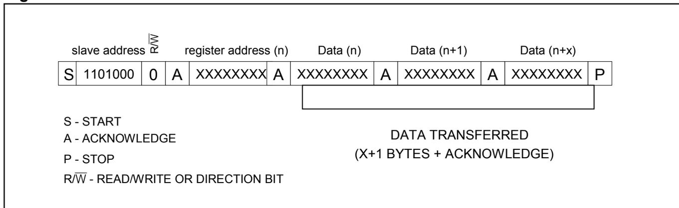
**Figure 9. Data Read—Slave Transmitter Mode**
