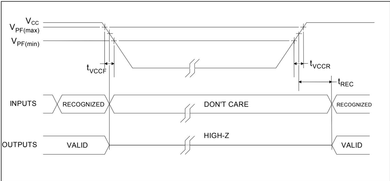
Figure 2. Timing Diagram
