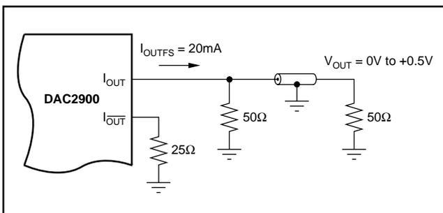
FIGURE 6. Driving a Doubly Terminated  $50\Omega$  Cable Directly.
