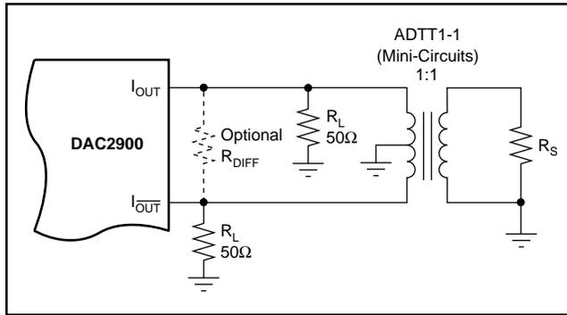
FIGURE 3. Differential Output Configuration Using an RF Transformer.
