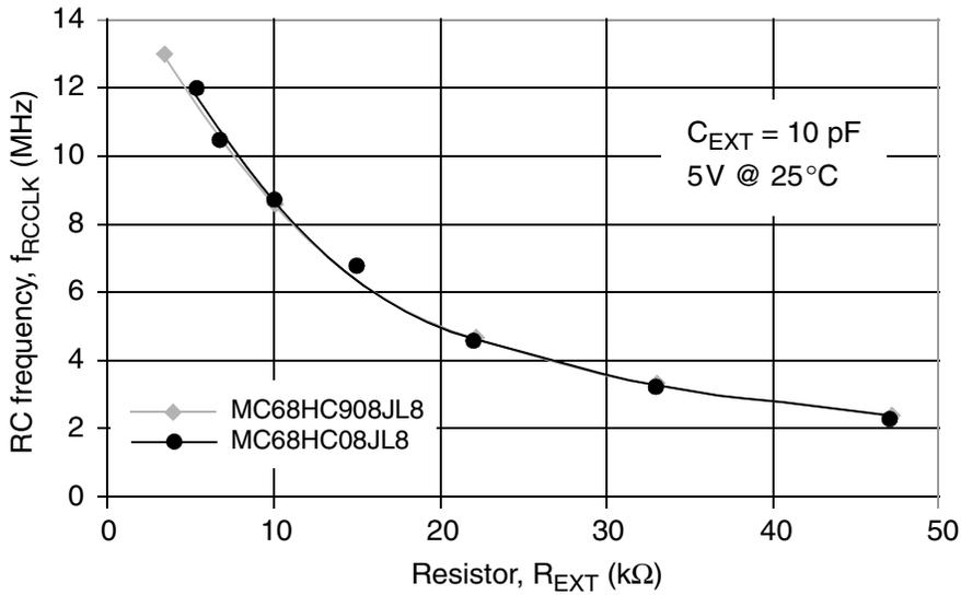
Figure 3. RC vs. Frequency (5V @ 25°C)
