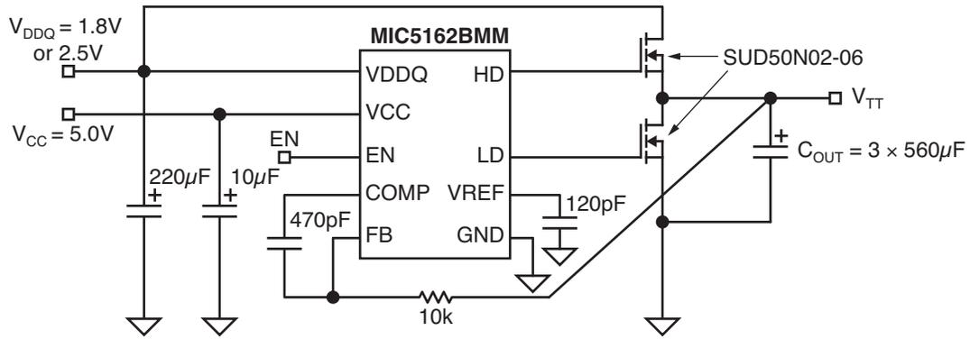
Figure 1. Test Circuit
