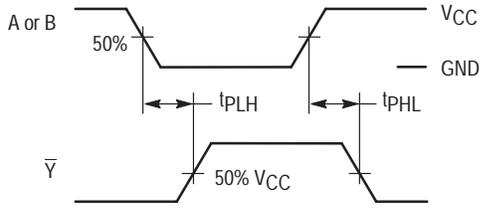
Figure 2. Switching Waveforms
