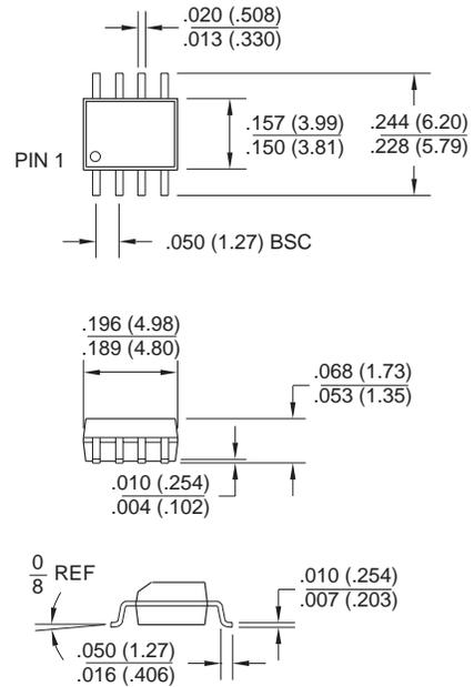
**8T**, 8-Lead, 0.170" Wide, Thin Small Outline Package (TSSOP) Dimensions in Millimeters and (Inches)\*
