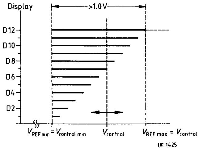
If a quartet does not need the full number of display diodes and if the first connected diodes shall be left luminous at full driving, bridges have to be inserted replacing the missing LEDs. Otherwise the first diodes of the quartet switch off when their display range is exceeded.
