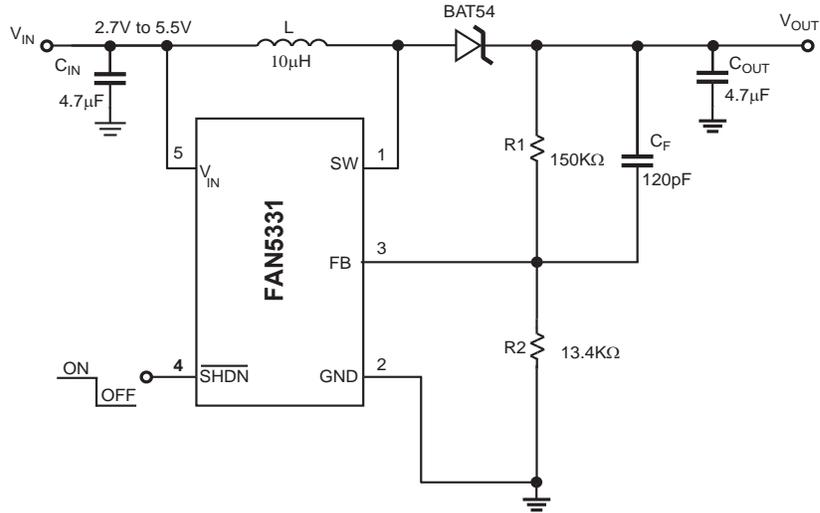
Figure 3. Test Circuit
