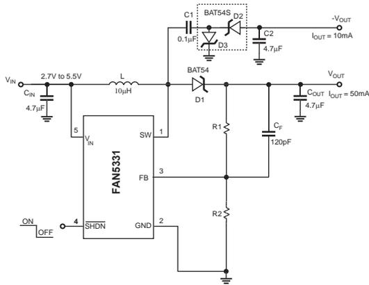
Figure 7. Dual ( $\pm$ ) Boost Converter
