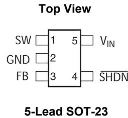
**Figure 2. Pin Assignment**
