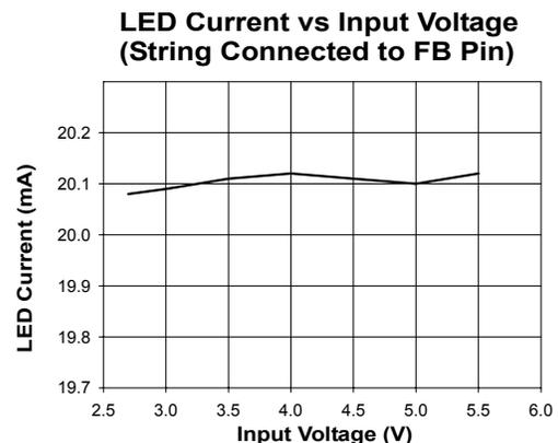
The feedback loop tightly regulates the current in the branch connected to FB pin, while the current in the other branch depends on the sum of the LED's forward voltages,  $V_{OUT}$  and the ballast resistor. The input and the output ripple is less than  $3mV_{RMS}$ , for load currents up to 40mA.
