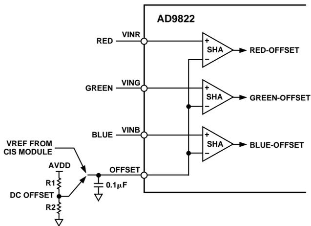
Figure 12. SHA-Mode Used with External DC Offset
