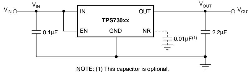
**Figure 16. Typical Application Circuit**
