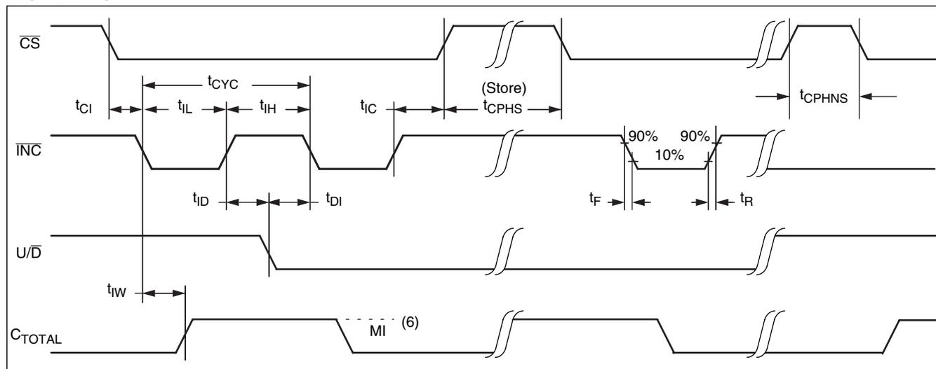
**Notes:** (6) MI in the A.C. timing diagram refers to the minimum incremental change in the  $C_{TOTAL}$  output due to a change in the counter value.
