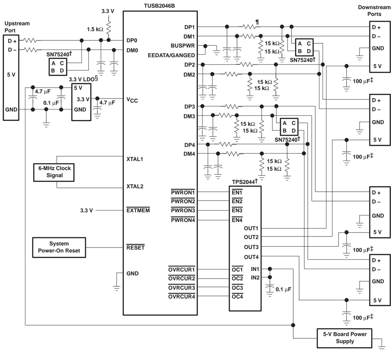
† TPS2042 and SN75240 are Texas Instruments devices. Two TPS2042 devices can be substituted for the TPS2044.
