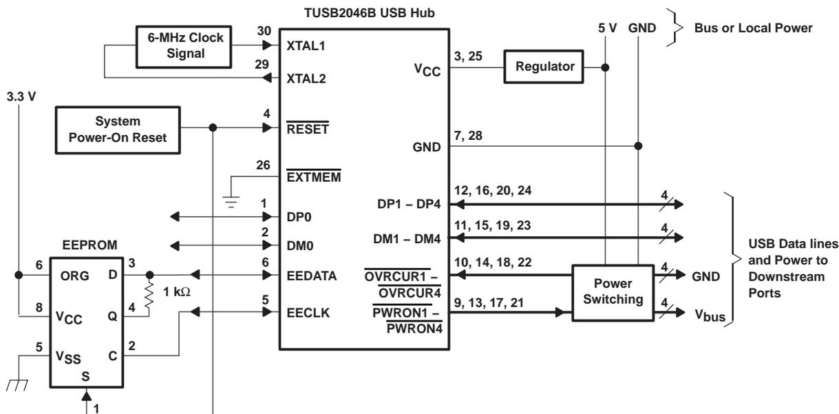
Figure 9. Typical Application of the TUSB2046B USB Hub
