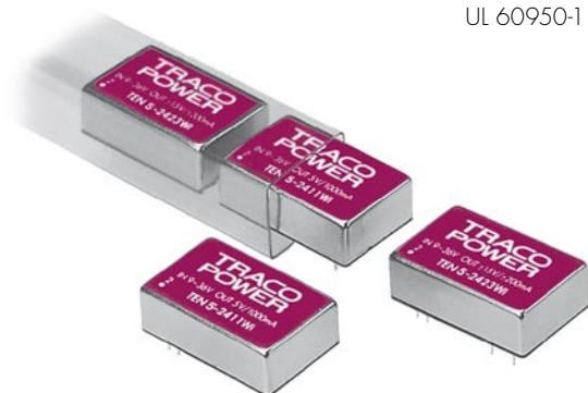
The TEN 5WI series is a family of high performance dc-dc converter modules with 5W output power, featuring ultra wide input voltage ranges of 9-36VDC or 18-75VDC. They come in a shielded DIP-24 metal package with industry-standard footprint.
