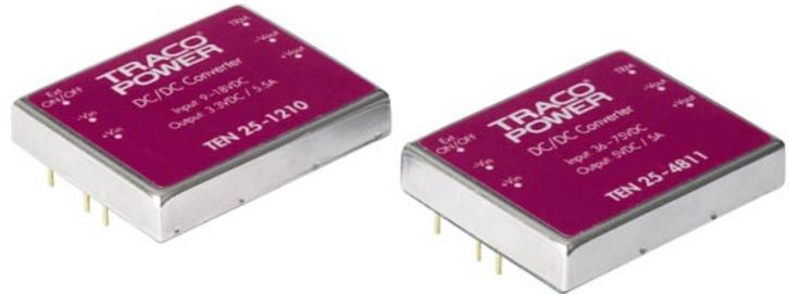
The TEN 25 series is a range of isolated DC/DC converters with high power density in a 51x41x9.5mm shielded metal case. All 18 models have a wide 2:1 input voltage range. The very high efficiency allows a safe operating temperature range of -40°C to +85°C. Other features are internal EMI-filter to meet EN55022, class A and remote On/Off. Typical applications for these converter modules are industrial electronics, communication systems, battery operated equipment and distributed power systems.
