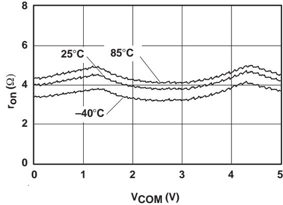
Figure 2.  $r_{on}$  vs  $V_{COM}$  ( $V_+ = 5V$ )
