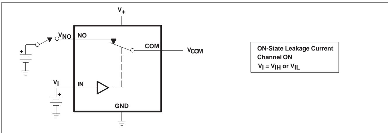
**Figure 15. ON-State Leakage Current ( $I_{COM(ON)}$ ,  $I_{NO(ON)}$ )**
