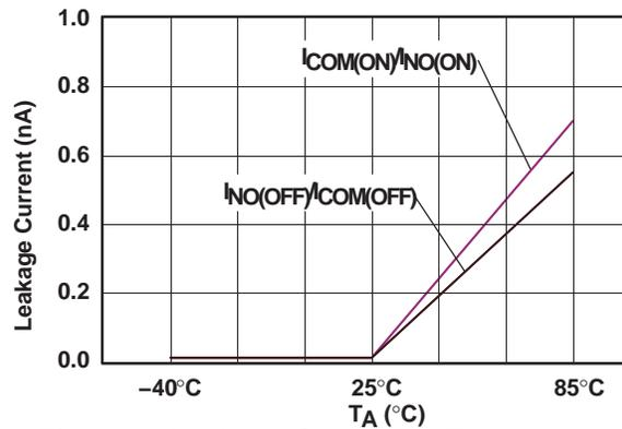
Figure 4. Leakage Current vs Temperature ( $V_+ = 5V$ )
