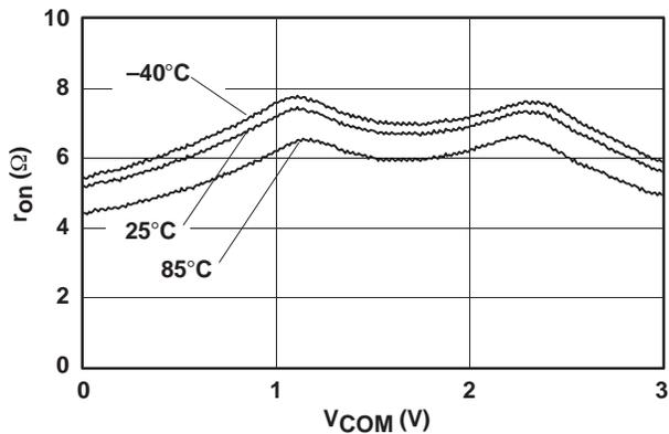
Figure 3.  $r_{on}$  vs  $V_{COM}$  ( $V_+ = 3V$ )
