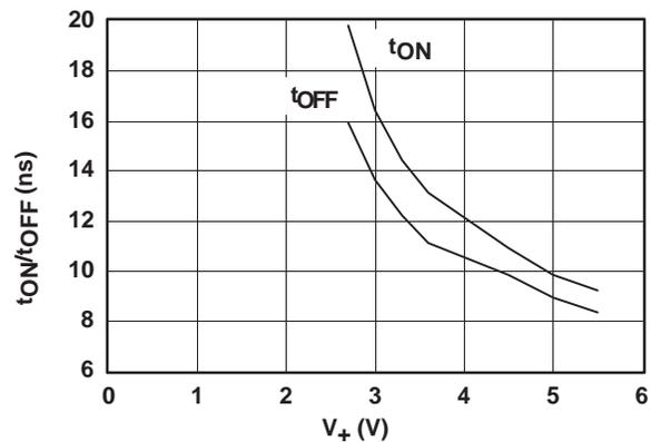
Figure 6.  $t_{ON}$  and  $t_{OFF}$  vs Supply Voltage
