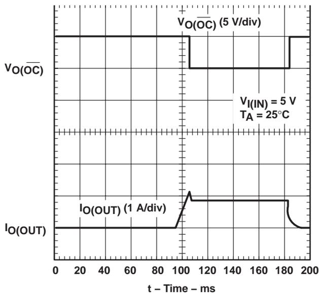
Figure 8. TPS2031, Ramped Load on Enabled Device
