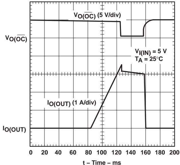
Figure 11. TPS2034, Ramped Load on Enabled Device
