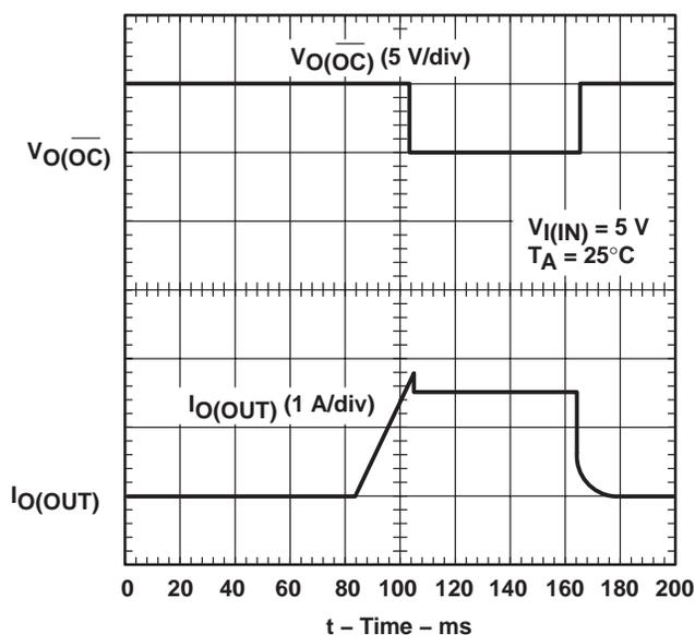
Figure 9. TPS2032, Ramped Load on Enabled Device
