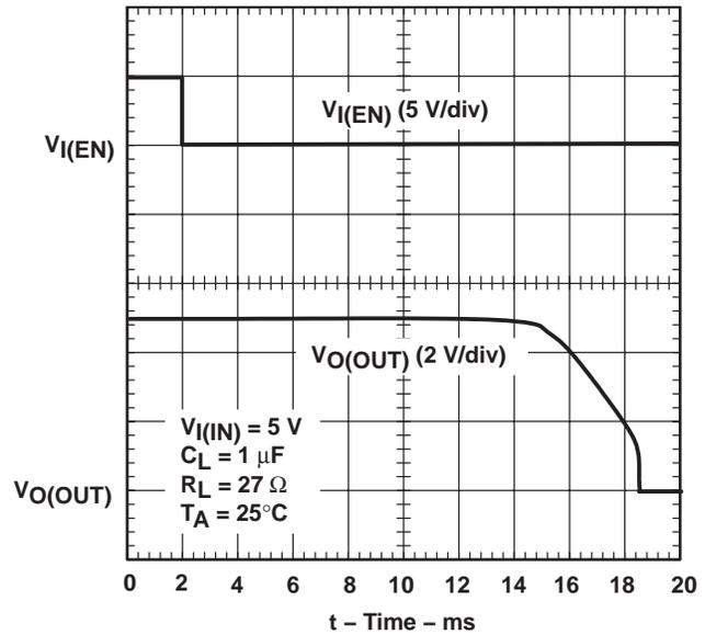
Figure 5. Turnoff Delay and Fall Time
