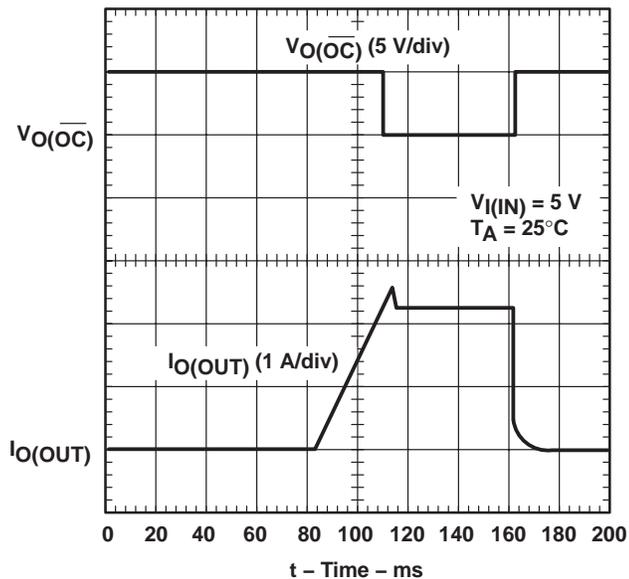
Figure 10. TPS2033, Ramped Load on Enabled Device
