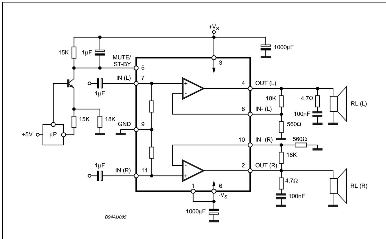
**ELECTRICAL CHARACTERISTICS** (Refer to the test circuit  $V_S = \pm 10V$ ;  $R_S = 50\Omega$ ;  $G_V = 30dB$ ,  $f = 1KHz$ ;
