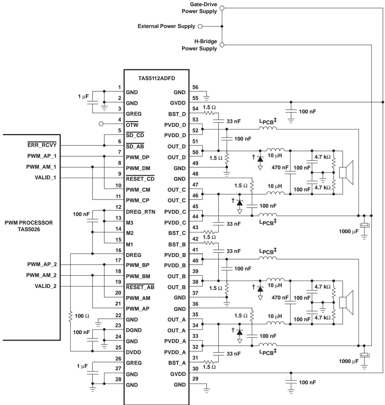
† Voltage suppressor diodes: 1SMA33CAT
