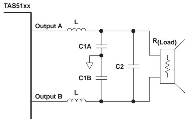
Figure 11. Demodulation Filter
